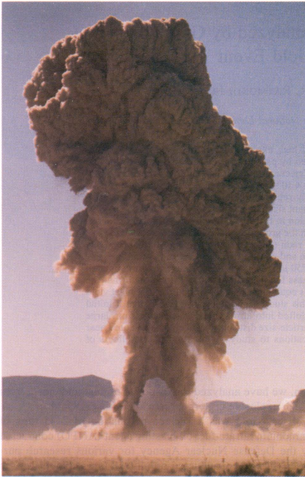
Plate 1. Photograph of the Misers Gold event, a burst of 2445 t of ammonium nitrate and fuel oil (ANFO) on an alluvial fan surface of the White Sands Missile Range, New Mexico, in 1989. Photograph is courtesy of the U.S. Army.
